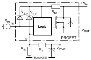
$R_{bb}$  = 120  $\Omega$  typ.,  $V_{Z,IN}$  =  $V_{Z,IS}$  = 66 V typ.,  $R_{IS}$  = 1 k $\Omega$  nominal. Note that when overvoltage exceeds 71 V typ. a voltage above 5V can occur between IS and GND, if  $R_{V},\,V_{Z,VIS}$  are not used.
