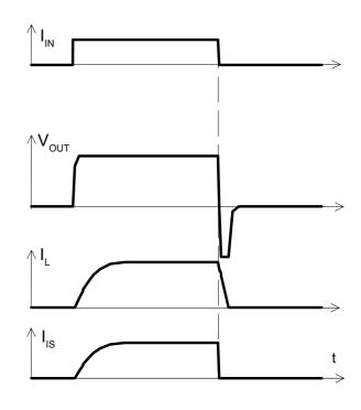
Figure 3a: Short circuit: shut down by short circuit detection, reset by  $I_{IN} = 0$ .
