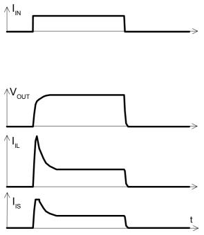
Sense current saturation can occur at very high inrush currents (see I<sub>IS,lim</sub> on page 6).
