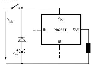
Note that there is no reverse battery protection when using a diode without additional Z-diode  $V_{ZL},\,V_{Zb}.$
