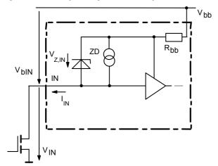
When the device is switched off ( $I_{IN} = 0$ ) the voltage between IN and GND reaches almost  $V_{bb}$ . Use a mechanical switch, a bipolar or MOS transistor with appropriate breakdown voltage as driver.  $V_{Z,IN} = 66 \text{ V}$  (typ).
