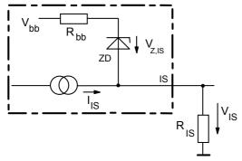
$V_{\rm Z,IS} = 66\,{\rm V}$  (typ.),  $R_{\rm IS} = 1\,{\rm k}\Omega$  nominal (or  $1\,{\rm k}\Omega$  /n, if n devices are connected in parallel).  $I_{\rm S} = I_{\rm L}/k_{\rm ilis}$  can be only driven by the internal circuit as long as  $V_{\rm out}$  -  $V_{\rm IS} > 5\rm{V}$ . If you want to measure load currents up to  $I_{\rm L(M)}$ ,  $R_{\rm IS}$  should be less than  $\frac{V_{\rm bb} - 5V}{I_{L(M)} / K_{\rm ilis}}$ .
