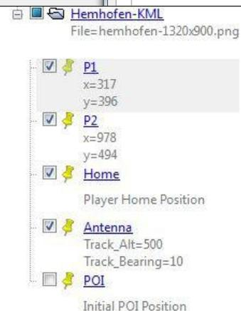
If you zoom in strongly enough in Google Earth, then the pin of the placemark can be positioned very precisely. The needle tip of the pin determines the desired location. The GPS coordinates of the placemark from GE is automatically determined and recorded
