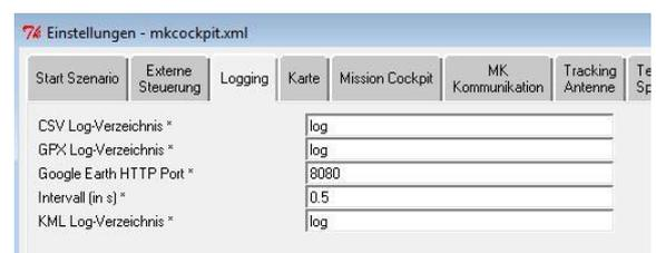
If the MK is "lost" by accident, then the server-based logging with the GPS positions can be very useful for finding the MikroKopter. In simulator mode, the logging is disabled.
