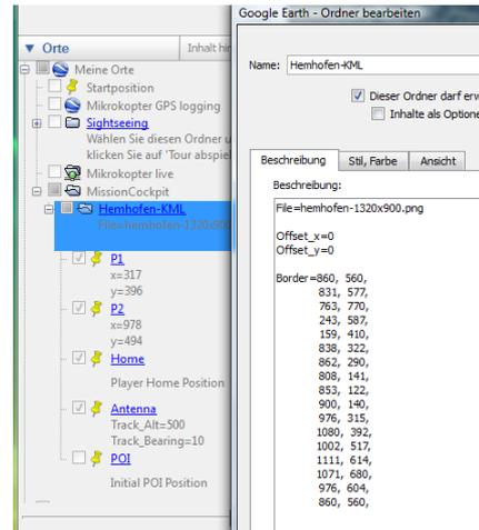
Under the folder create placemarks for the two calibration points **P1**, **P2**, and optionally for the **Home**, **Antenna** and **POI** location.
