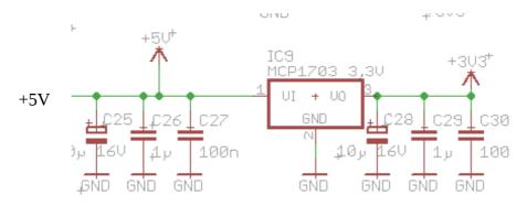
Creating After the assembly of this part of SJ1 pin 1 meter and turn on voltage (see above). Alternatively, one can also measure where the 3.3 V Displaypin 34.
