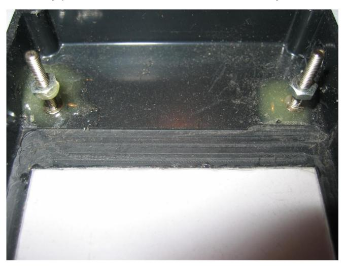
Here you can see also an alternative for fixing the circuit board, if one is inclined to do in the case screws on the back side and front view without screws.
