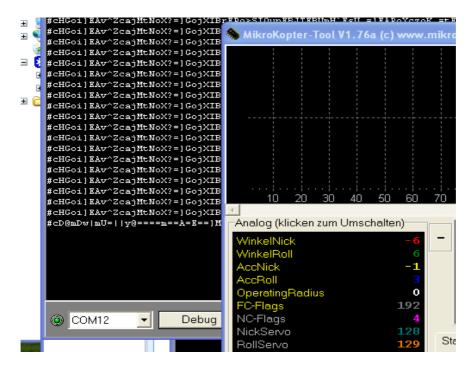
Once this is configured, you do not need activate the Bluetooth manually. In the moment when the MikroKopterTool used when starting the same COM port, the connection to the PKT is established automatically.
