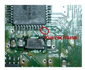
5. BTM222 LED2 does not blink. Reason: solder bridge between pin and feedthrough BTM222.
