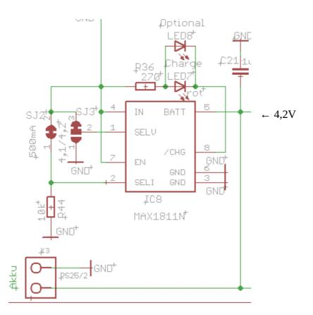
Connect USB cable to PC, now at the output of the MAX1811 should approximately 4.2 V can be measured. Then remove the USB cable again.
